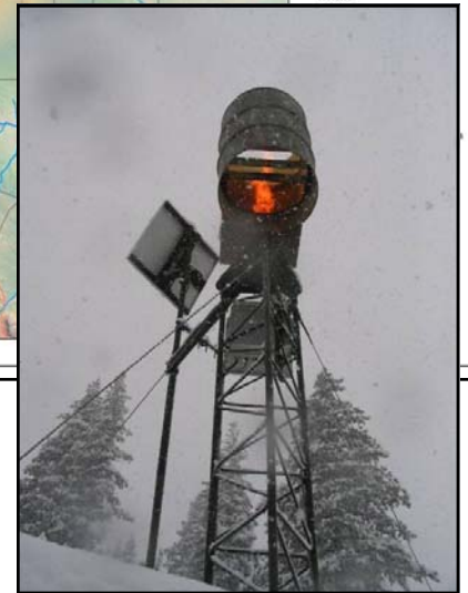
A Colorado Water Conservation Board map shows areas of focus for weather modification. At right is a cloud seeding generator in action. Details, page 2
